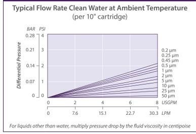
The micron ratings shown at various efficiency and beta ratio value levels were determined through laboratory testing, and can be used as a guide for selecting cartridges and estimating their performance. Under actual field conditions, results may vary somewhat from the values shown due to the variability of filtration parameters.
